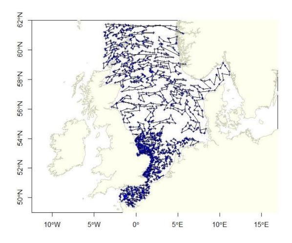
Figure 11. Salesman travelling problem applied to the proposed joint monitoring programme The route shown is the minimal route to link all the stations following the shortest track. The algorithm is also used to calculate the number of total nautical miles. It assumes that one survey vessel visits all stations, without visiting any harbour.
