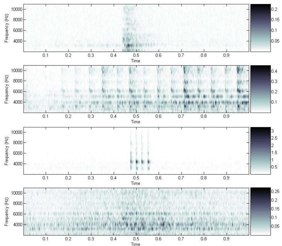
*Figure 8.12 Sonograms of regions of interest of several more typical non-bird sounds on the metmast, that were also identified correctly as non-bird sounds by the automated system. Bar on the right indicates signal strength. Top: metal door slam of container; second from above: trembling floor plate; third from above: raindrop falling with vibrating plastic protection sheet of the microphone; bottom: a typical large wave breaking on the post of the metmast.*
