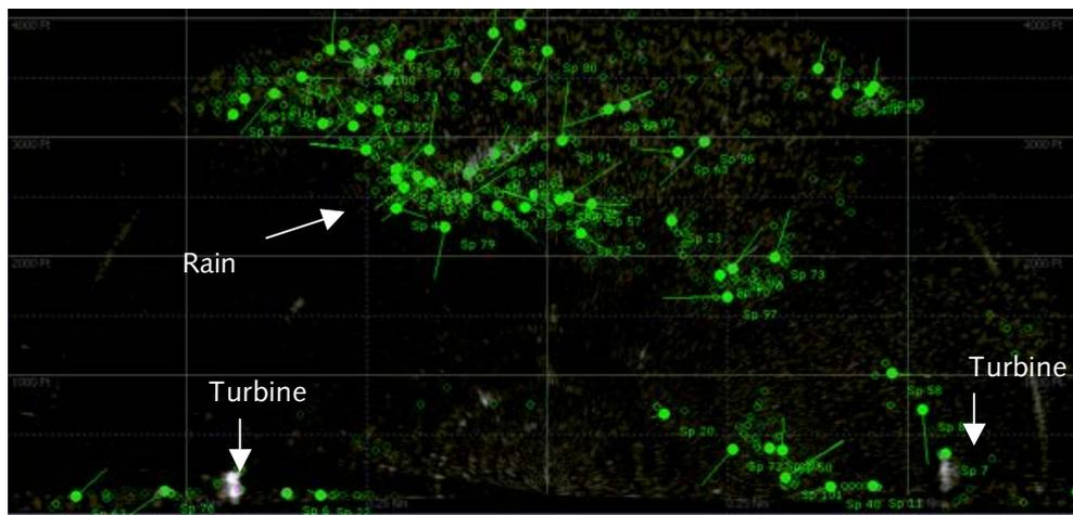
Figure 7.7 Radar images from the Merlin screen of the vertical radar, taken during a rain shower. Rain showers passing over the area were detected by the radar and tracked by Merlin. Two turbines are in the picture as well.
