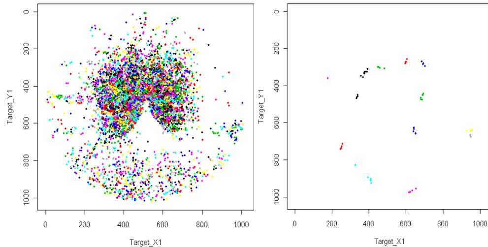
Figure 6.24 Sea clutter recorded on June 3 2009 during 5 minutes. Data before (left) and after filtering (right). Each echo is a symbol, echoes belonging to the same track have the same colour.
