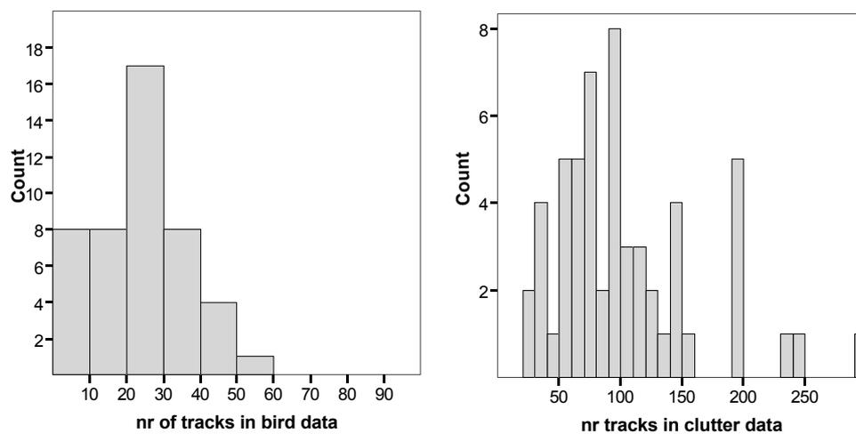
Figure 6.11 Frequency distributions of the number of tracks (echoes) that Merlin recorded per scan at times when birds were visible (left panel) and at times when only sea clutter was visible on the horizontal Merlin screen. Note the difference in scale. When birds were visible, the number of echoes per scan was lower than 60.
