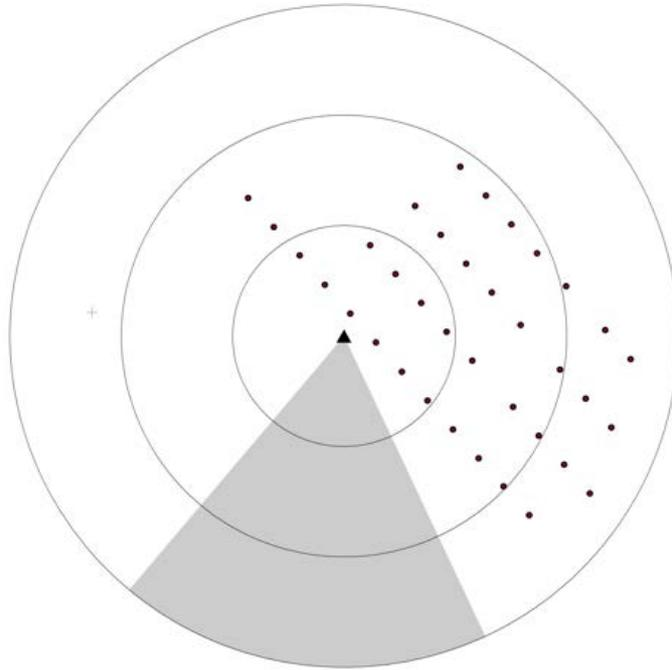
*Figure 5.5 Area covered by the radar. Range is set at 3 NM, which includes the entire wind farm (rings drawn at 1 NM intervals). Turbines are shown as 36 bullets, the metmast with the radar is shown as a triangle in the centre. The sector that would be obstructed by the metmast structure was blanked and is shown as a grey triangle to the south of the radar.*
