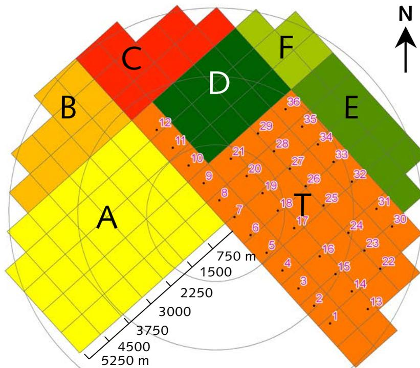
Figure 9.13 Classification of areas (blocks) used to analyse detection loss in horizontal radar data due to interference from turbines. Scale indicates distance of grid cells from radar in m.
