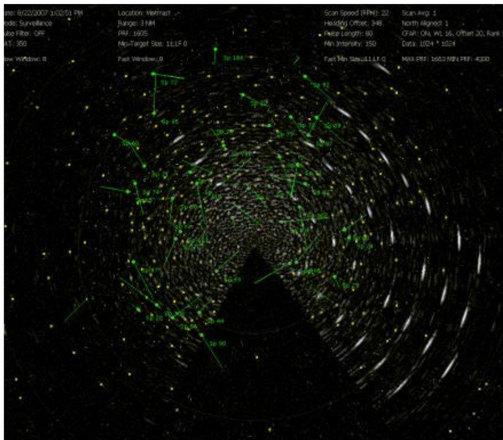
Figure 6.6 Merlin tracking waves in a wide area around the radar.
