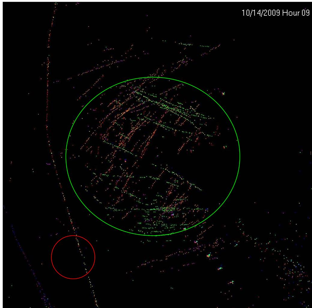
Figure III.1 Trackplot images of raw radar data from the VTS radar at turbine 21 on the 14<sup>th</sup> of October 2009. Bird tracks (green circle) as well as the track of a ship (red circle) can be seen.
