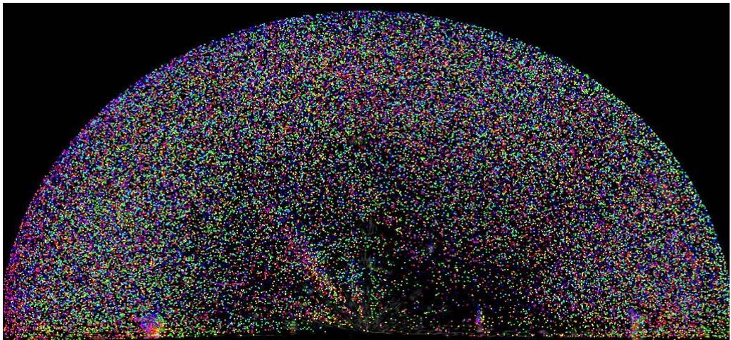
Figure 7.13 Trackplot picture of Merlin screen of one hour on the 5<sup>th</sup> of November 2009 showing rain clutter.
