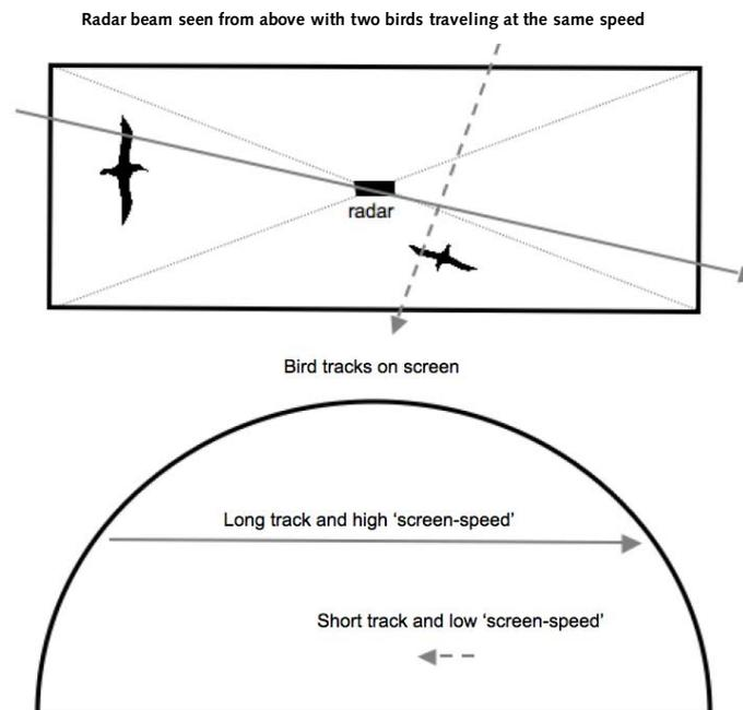
*Figure IV.1 Schematic overview of two birds flying with the same speed through the radar beam giving different 2D trail lengths and echo speeds in Merlin. 2D speed and distance thus provides information on actual heading.*
