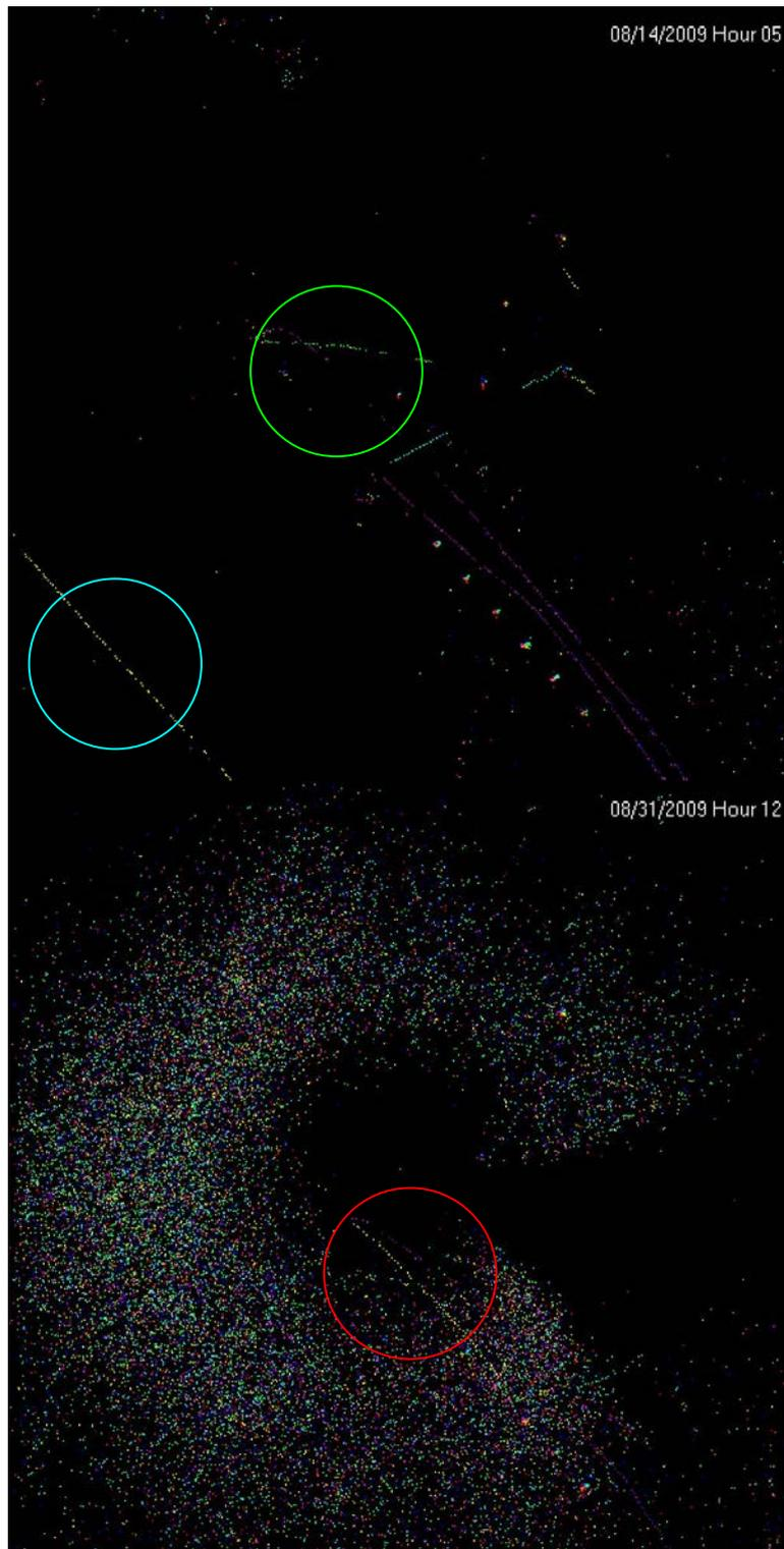
Figure III.2 Trackplot images of raw radar data from the VTS radar at turbine 21 on the 8<sup>th</sup> of August 2009 (wind: east 4 Bft. & 31<sup>st</sup> of August 2009 (wind: south 4 Bft). A supply vessel arriving and departing a turbine is visible (red circle) as well as a ship leaving IJmuiden harbour (blue circle). Some bird tracks were also visible (green circle).
