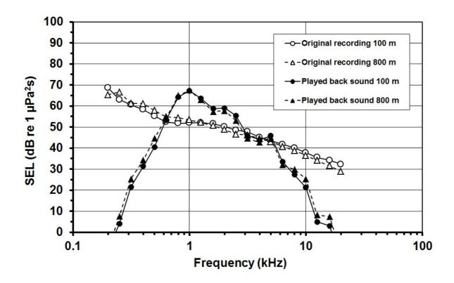
FIG. 3. The 1/3-octave band spectra of the SEL (over the 90% energy duration of the sounds) of the original and played back pile driving sounds in the pool. All spectra are scaled to the same total unweighted broadband SEL of 74 dB re 1  $\mu$ Pa<sup>2</sup>s in the 200 Hz to 20 kHz 1/3-octave bands.
