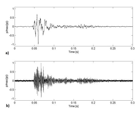
FIG. 2. Waveform of a single pile-driving sound recorded at 800 m from the pile driving site (a), and of the played back sound in the pool (b). The amplitude of the sound pressure is scaled to the maximum absolute value of instantaneous sound pressure.
