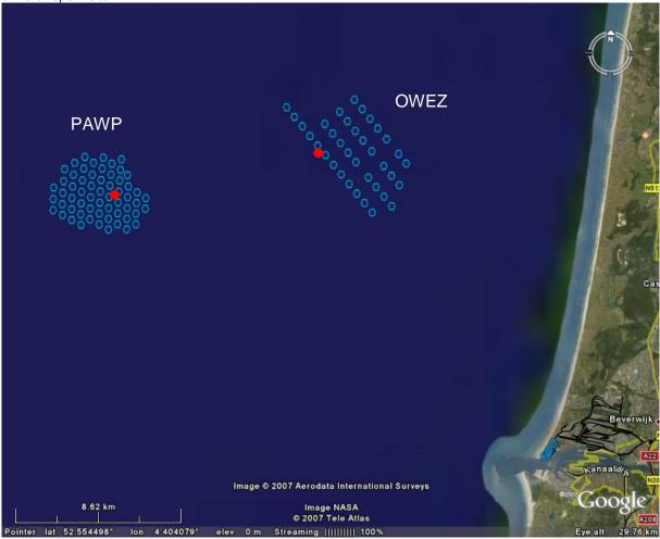
**Figure 1.** Location of the 36 OWEZ turbines (right) and the 60 PAWP 60 turbines left, to the northwest of the port of IJmuiden (lower right). In addition to the turbines, OWEZ has a 116 m high met-(meteo)mast situated centrally on the seaward (SW) side of the wind farm, and PAWF has a transformer platform within the wind farm. Image from: http://home.planet.nl/~windsh/Offshorelocaties.jpg. The red dots (added to the original picture) represent the OWEZ metmast and PAWP transformer platform.
