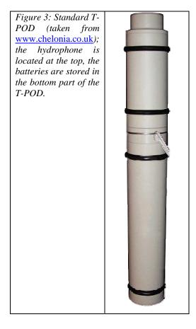
Comparison of T-POD recordings with simultaneous visual tracking of porpoises with theodolite show that the effective detection distance is between 100 and 200 meters (with a maximum detection of around 500m). Of 37 animals observed closer than 100 m from the T-POD, 81% were registered by the T-POD. Of 34 animals that came within 100-200 meters, of the T-POD, 31% were recorded by the T-POD (Tougaard 2008).
