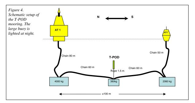
Each T-POD was deployed between two large buoys, of which the larger was equipped with a yellow warning lantern. Furthermore, the experimental setup was proclaimed on VHF-radio regularly by the local authorities.
