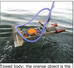
Towed body; the orange object is the 38 kHz transducer.
