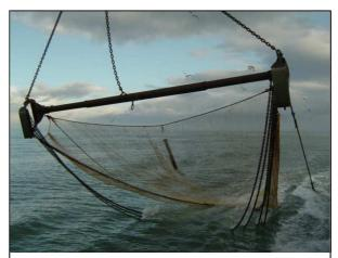
One of the 6m beam trawls used during the demersal survey. Attached to this beam is the 20 mm net. In the middle of the net, the CTD device is visible (Grift 2004).
